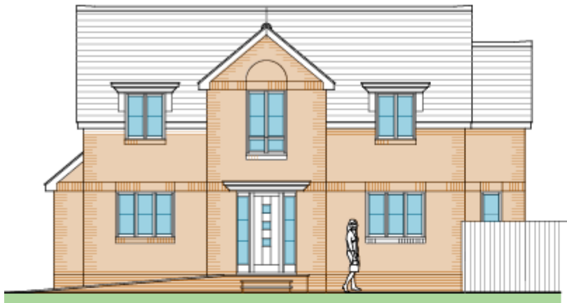
PROPOSED NORTH ELEVATION
